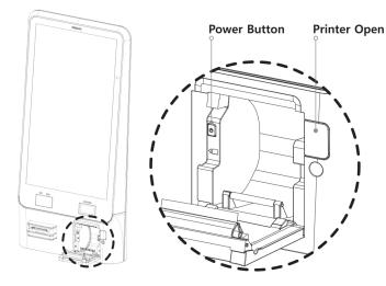
Step 1. Press 'OPEN' Button to open printer cover.
